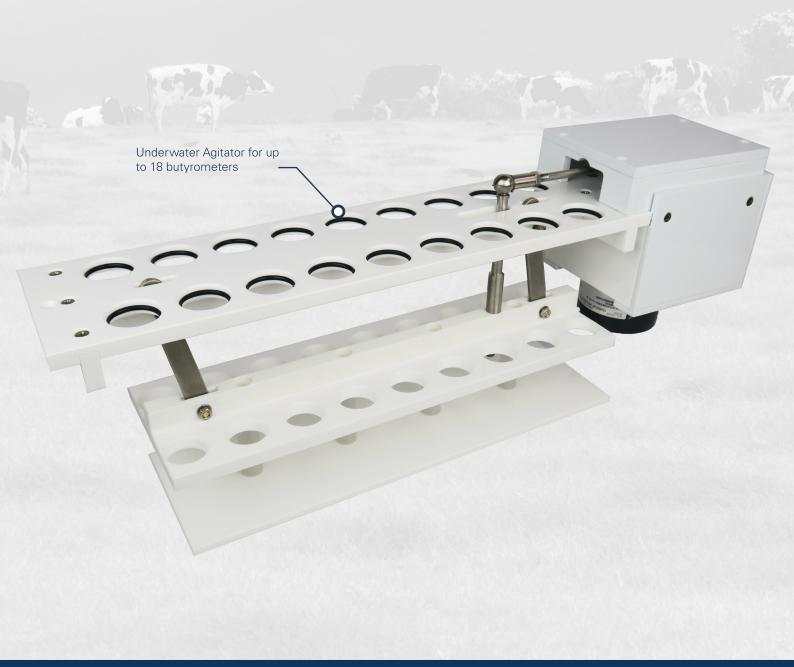
The Aerne Analytic Underwater Agitator is used for an equal intermix of samples in butyrometers at a constant temperature. It works with high precision and safety standards. The agitator can be inserted in waterbaths that have an effective space of 39x25x20cm and 30x15x20cm. The housing
