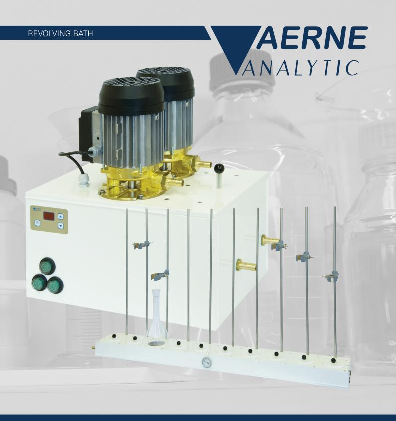
The Aerne Analytic Series Baths for explosion-proof areas are used for extraction or distillation with ether or other inflammable mediums. The heating occurs indirectly by a circulator which is positioned outside of the danger area. The Series Baths are equipped with openings for round or flat-bottomed
