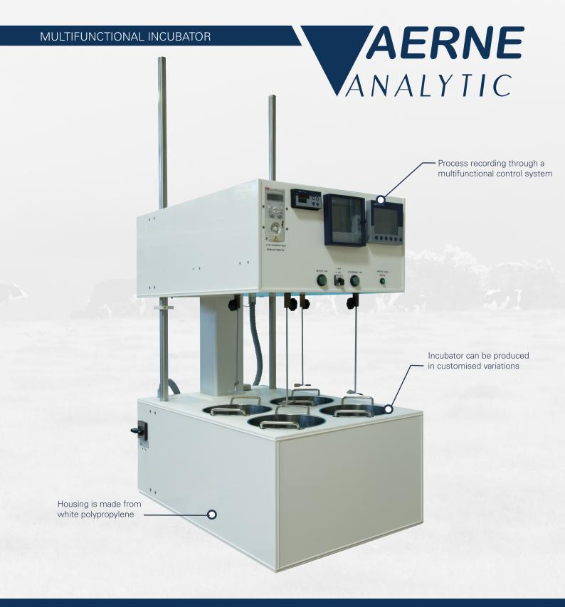
The Multifunctional Incubator, which is made from white polypropylene, is used for culture of bacteriums or yeast cultures, for example for the dairying. The incubator works with an individual program for the temperature and time (pasteurisation, incubation, cooling), an adjustable agitator with lifting column that is
