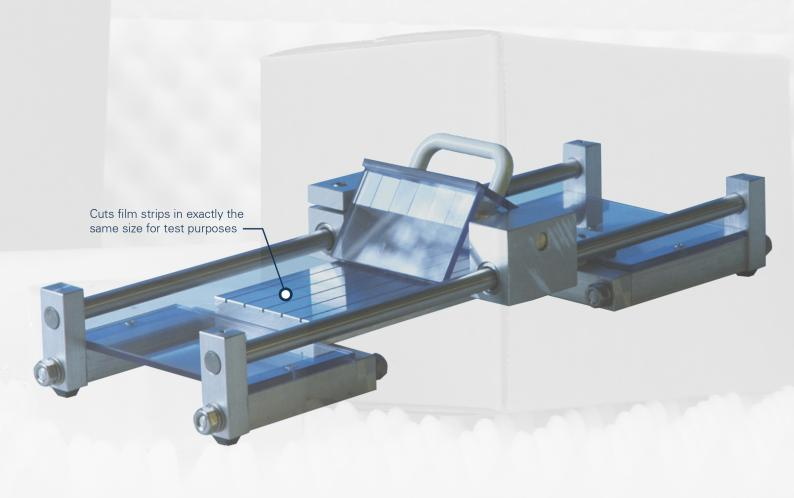
The Aerne Analytic Foil Cutter is used to cut film strips in exactly the same sizes. The strips are necessary in the quality assurance in film manufacturings. By means of for example tensile tests the suitability can with the help of a stress-strain diagram be analysed and determined. The cutter works
