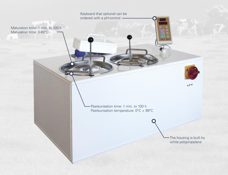
The Aerne Analytic Incubators are used for raising bacteria or yeast cultures, e. g. acidification cultures, in the dairying. Optimal results can be reached by programming individual processes. Beause of the very good heating isolation of polypropylene the Incubator can be built in a single-walled type
